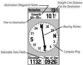
The Navigation Page provides active guidance with a rotating compass ring that shows your course over ground (track) while you're moving and a bearing pointer to indicate the current direction to your destination (bearing) relative to the course over ground.
