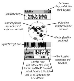
The Satellite Page provides a picture of satellite signal tracking, tells you when the unit is ready for navigation, and shows your location coordinates.
