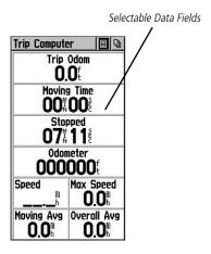
The Trip Computer Page displays up to eight different types of navigation data and are user programmable. Each data field is selectable and can contain one of many data information options. The default settings for these fields are shown in the illustration.
